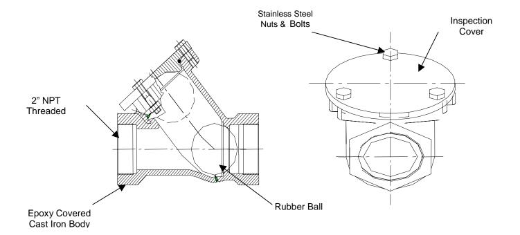
Armstrong check valves are designed for use with polluted liquids of a variety of viscosities and chemically aggressive liquids. The mechanism consists of a ball shaped sinking shutter which guarantees an excellent seal and passage of solid bodies with no risk of clogging.
